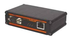
External RS232 to TCP/IP converter for UPS and STS
